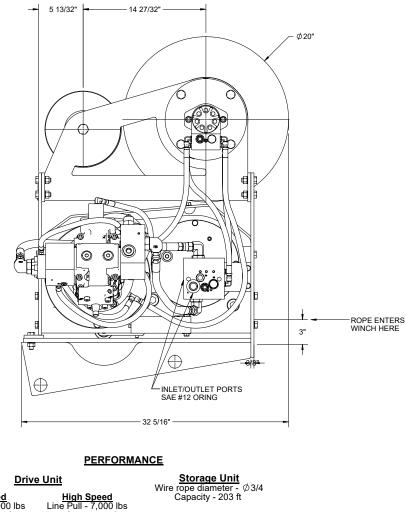
Low Speed Line Pull - 35,000 lbs Line Speed - 20 fpm
